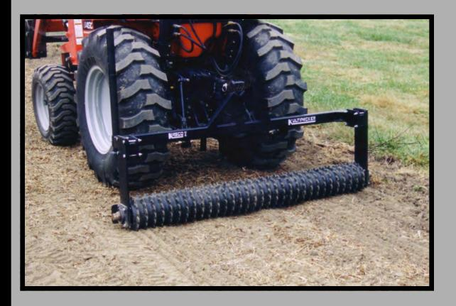
Heavy Duty Culitpacker Roller to Firm and Level Soil after Seeding
