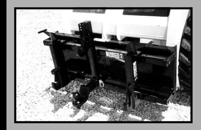
The Switch Hitch Allows You to Use 3-Point Implements on Your Skid Steer Loader.
