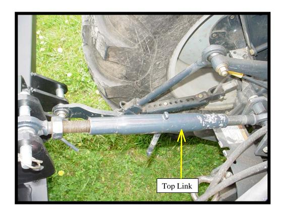
Depth Control is determined by One Measurement 1) The front slicing disc can be adjusted by the top link. Shortening the top link will put more depth and pressure on to the slicing discs; lengthening the top link will remove depth and pressure from the slicing discs.
