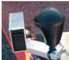
Rocker switch allows the operator to control grapple movement with the touch of a finger.
