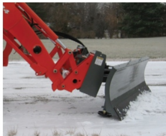
Adjustable skid shoes are standard
