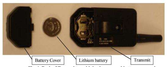
Fig. 4: Back of Transmitter with back cover and battery removed
