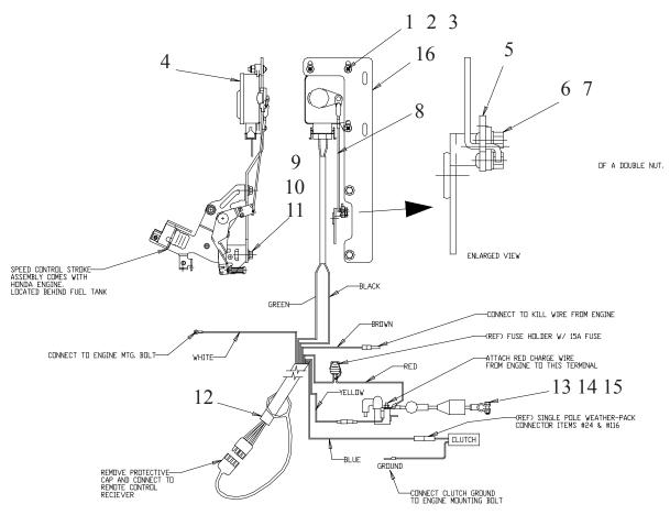
DETAIL, WIRING & THROTTLE ASSEMBLY SCALE .375
