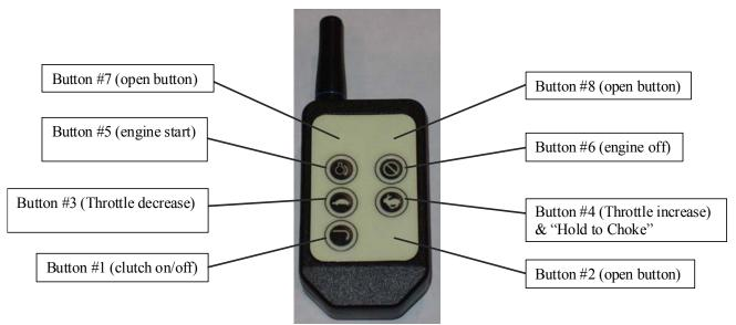
Fig. 1: Transmitter Front Button Assignments
