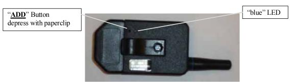
Fig. 2: Transmitter Back Button Assignments
