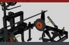
The greenhouse plastic mulch layer, pulls the irrigation belt and places the plastic for the padding in one step.
