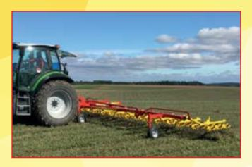
The AS Series Tined Weeders efficiently pull out weeds that have germinated, leaving them on the soil surface to wither. Approximately 90% of germinated weeds are stopped in their tracks.
