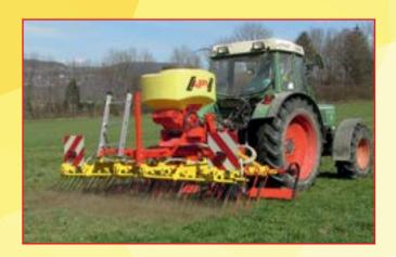
The GS 300 M1, a compact cultivation implement, has a working width of 9.10 ft. It can be used by small tractors starting at 27 hp. Perform up to six tasks with the GS with only one pass, saving time and energy. It also reduces soil compaction and fuel consumption. The GS 300 M1 can be used with Pneumatic Seeders with electric fans such as the PS 120 M1, PS 200 M1 and PS 300 M1.
