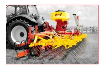
The impressive all-rounder GS 600 M1 is suitable for the efficient treatment of grassland due to the larger working width of 19.7 ft. It is characterised by a high tilt adjustment and can also be used in difficult terrain. You can combine up to six tasks with the GS 600 M1. It can be used with Pneumatic Seeders with electric fans, hydraulic fans or PTO shaft fans PS 120 M1, PS 200 M1 and PS 300 M1.
