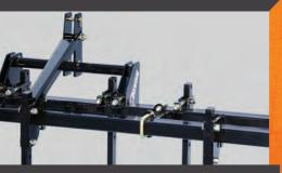
Easy adjustment for desired cultivation width, just slide the shanks on the tool holder bars.
