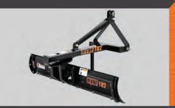
End plates allow rear blade to hold in material for filling.
