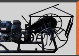
Wire guide provides even wire distribution, and keeps hands safely away from wire.
