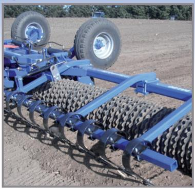
The hydraulic cracker board is mounted to the main frame by easily fitted arms. The cracker board tines are of 80 x 10mm spring steel with specially designed points. When the machine is used for rolling the cracker board can be raised out of work.
