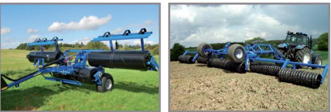
The simple operation of folding/unfolding of the Compact rolls and adjustments for the cracker board or mole hill board are all controlled hydraulically from the tractor cab.
