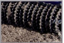
The **Crosskill ring** is a cultivation ring, which leaves a porous surface, with less risk of erosion and sand drift. Every other ring is mounted loosely onto the shaft, which ensures that the roller is very good at keeping itself clean. The crosskill rings are also very robust against stones. It is also suitable for rolling in germinated areas.
