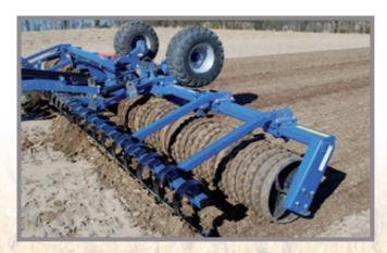
The heavy duty XL frame can be fitted with a hydr. Cracker board or a mole hill board.
