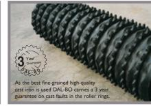
The **Cambridge/breaker ring** is recommended for rolling in germinated areas and in grass fields. The toothed rings break the surface so that the roots are aerated. The lightly waved large rings ensure that the roller does not block in loose soil. The new rounded profiles protect the plants and make the rings less vulnerable when driving into stones. Cam, welled and smooth rings are also available.
