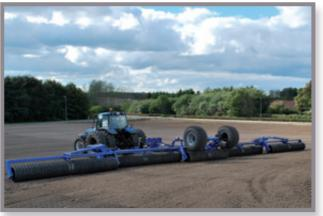
Compact hydraulic rollers with working width 12.30 - 18.30 m
