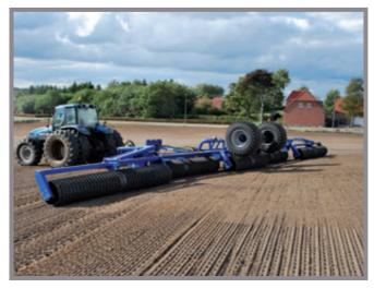
The 18.3m Compact is the new flagship model in the 5 section range. Fitted as standard with centre bearings to each section, rubber suspended bearings mounted to the ends of the CRMO4V high quality steel axles and large 600/50-22.5 wheels ensure the best possible quality is guaranteed.
