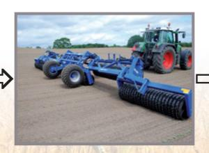
The folding/unfolding is done from a stationary position. Once the roller has been completely unfolded it can be lowered. At this stage the wheels will smoothly lift clear of the ground.
