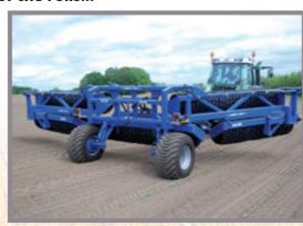
First the wing sections are lifted out of the transport locks and then the unfolding of the inner sections.
