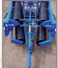
The Compact 5 section roller has a 3m transport width.
