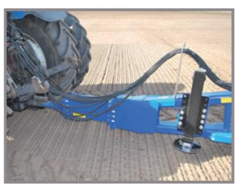
On machines 14.3m and wider a hydraulic jack is fitted as standard. The extended drawbar makes turning so much easier.
