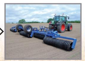
Then, via the accumulator you pressurize the side sections so that an even soil pressure is applied across the full working width.
