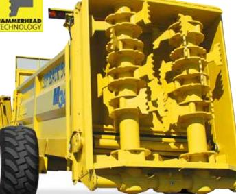
The paddles are interchangeable, reversible and can be easily replaced by removing a single over sized pin - without cutting or welding. These induction hardened chrome pins are sealed at either end by polymer bushings creating a completley greaseless
