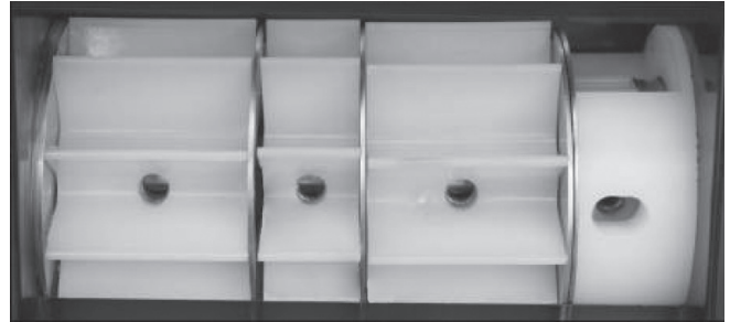
Low compression: Insufficient side pressure creates gaps.
