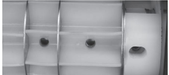
High compression: Wheel rib edges become curled/wavy.
