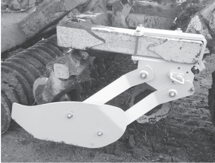
Dirt deflector is located on outer edge of the right wing frame. Extension is required for ProTill 40 Controlled Traffic Models. (Note: Previous Deflector Plate shown)
