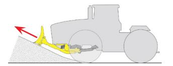
When an adjustment needs to be made by the operator, fast blade response time is necessary. The Degelman Silage King is mounted with only one pivot point, making the response time as quick as possible. This radial lift design makes it easier to push, carrying loads **UP** the pile, rather than **INTO** the pile.
