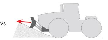
The parallel lift approach, used by competitors, not only pushes silage **INTO** the pile, but also contains up to 6 different pivot points, causing slow blade reaction time when an adjustment is made by the operator. This outdated approach can cause numerous headaches when pushing silage.
