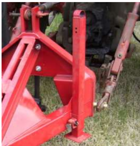
Figure 10: GA-700 Attachment to a Category 2 Three Point Hitch
