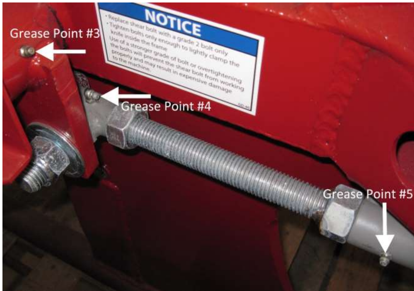
Figure 17: Grease Points on Packer Wheel Adjustment Rod
