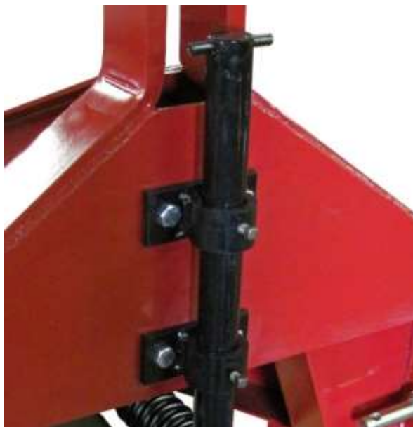
Figure 7: Assembled Coulter Shank
