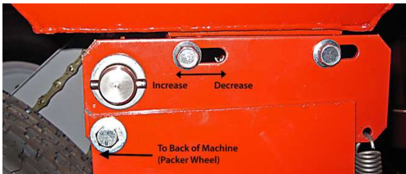
Figure 11: Adjusting Rate of Bait Application
