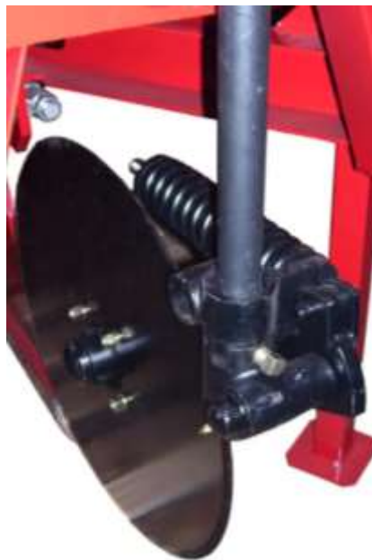
Figure 9: Completed Couler Assembly
