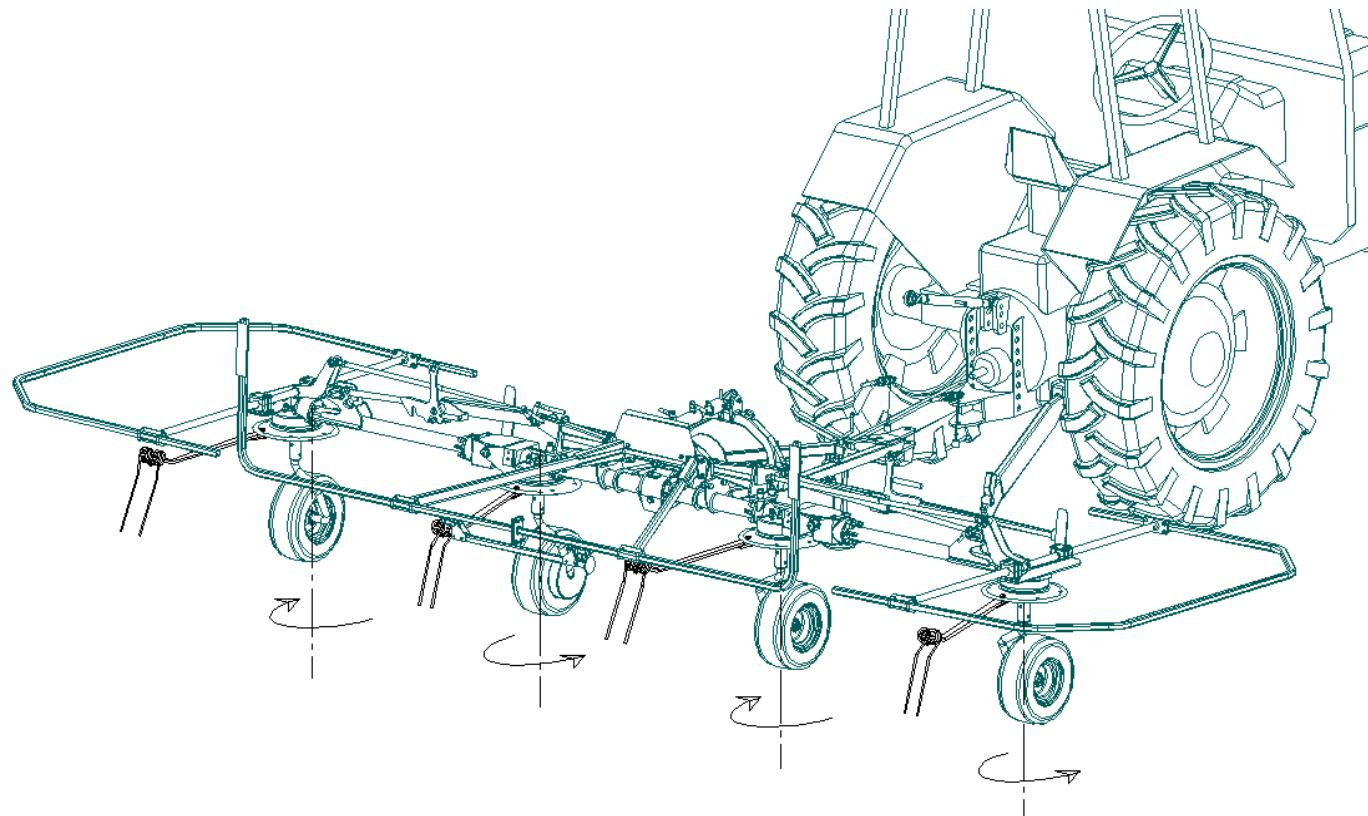
**Correct positioning of tines**
