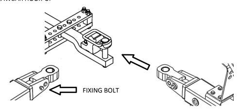
Keep the pull block on horizontal position tightening the fixing bolt. Be sure to loosen the bolt before operating.
