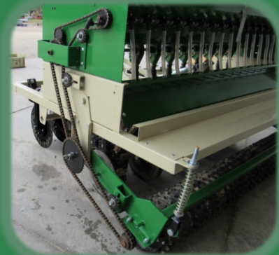
High Precision Ground Drive Seeding System. You Stop-Seeds Stop Flowing!
