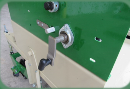
Simple Highly Accurate Fluted Seedcup Adjustment System
