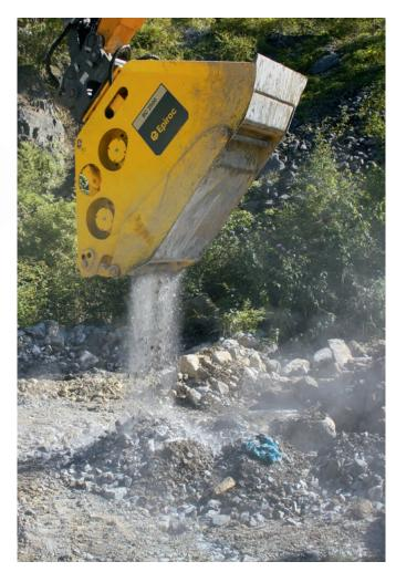
Our Bucket Crushers combine low maintenance and high performance. On-site crushing also means less transportation and dumpsite costs.
