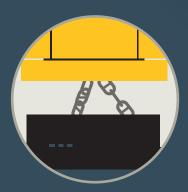
Built-in **generator with advanced control technology** provides faster material pick-up by a quick magnetization with impulse excitation and material release by automatic demagnetization with counter voltage and sequence pulsation.
