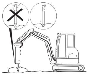
■ The hydraulic breaker or the working tool is not to be used as a lifting device. When lifting heavy components use the hook on the carrier arm.
