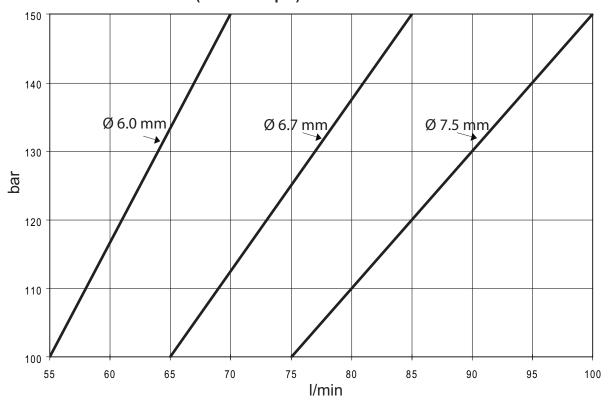
SB 452 Tunnel is delivered with restrictor Ø8.7 for 110 bar (1595 psi) operation. As an option, restrictor Ø7.5 for operation at higher pressure, is available.
