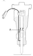
Lubricate the working tool's shank plentifully during all upward operations. The bushing and the working tool must be lubricated so frequently that dirt cannot penetrate into the hydraulic breaker.
