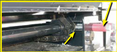
The idler apron shaft assembly features 6-tooth machined steel sprockets with bronze idler bushings. Shown with shield open.
