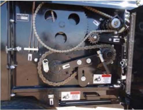
Quick Release Cross Conveyor Clean-Out Pan Shown with shield open.
