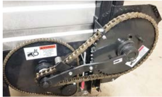
QUICKLY CHANGE FROM FRONT TO REAR UNLOAD Changing the drive system from front to rear unload is as simple as removing the drive pin from the front drive sprocket and placing it in the rear drive sprocket. Shown with shield open.
