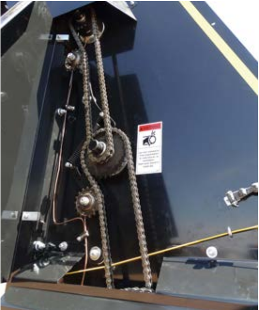
Spring Loaded Tighteners on Beaters. Shown with shield removed.
