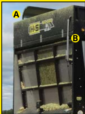
The Big Dog features an electric actuator (A) and roof hood (B).
