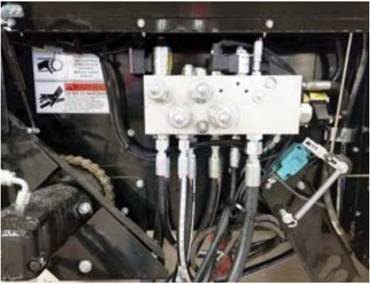
HYAULIC MANIFOLD A hydraulic manifold with quick couplers allows you to change from front unload to rear unload quickly. Shown with shield open.
