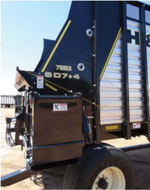
CROSS CONVEYOR EXTENSION A 24" Hydraulic Fold Cross Conveyor Extension is standard equipment on all 7200 series models.
