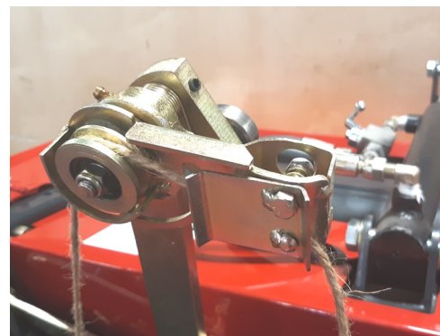
Twine Tensioner #2 (end of binding arm)
