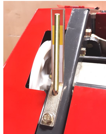
Bale Chamber Indicator at max.
