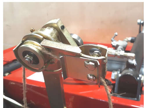
Twine Tensioner 2 (end of binding arm)
