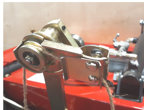
Twine Tensioner #2 (end of binding arm)
