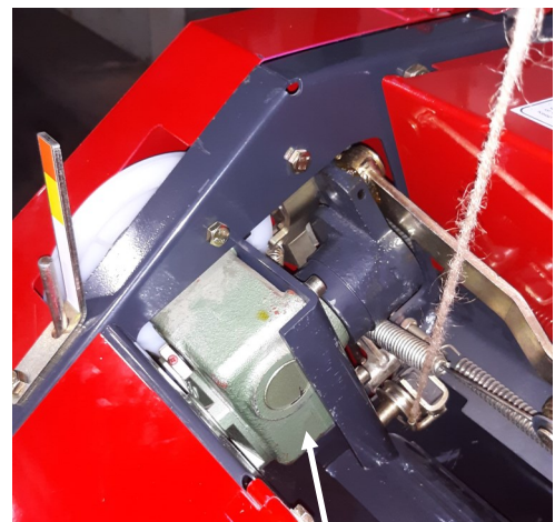
Binding Arm Gearbox
