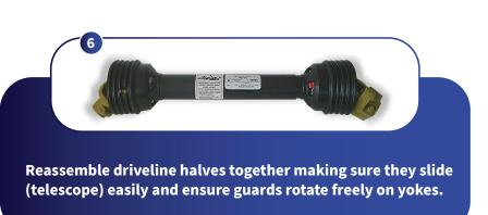
**EXAMPLE:** If overall replacement driveline length dimension is 48" (See A), and your existing overall driveline length dimension is 42" (See B), the amount to shorten EACH driveline half would be 6". Your driveline is now ready to reassemble and use.
