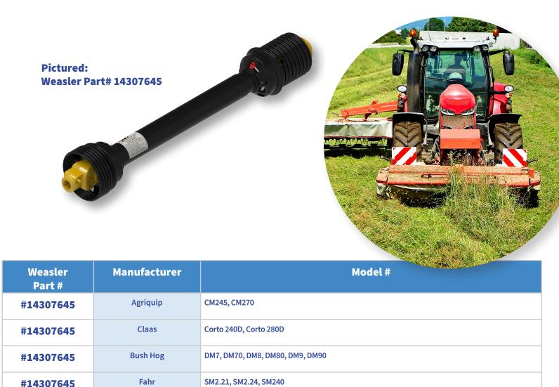
**NOTE:** Before installing verify correct end yoke and overall driveline fitment. It may be necessary to cut the driveline to length to fit your specific application. Verify the length by ensuring that sufficient overlap of the profile tubes exists in all working positions without the possibility of bottoming out. Safety decals must remain intact if driveline has been modified.
